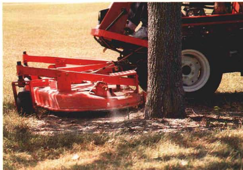
After mowing around the trees, a flick of a switch applies an application of non-selective herbicide to any remaining vegetation.
