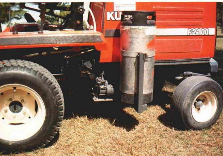
Through some innovative engineering, an out-front rotary mower can be transformed into a highly specialized spray rig. Canisters are mounted on the back of the mower body to carry herbicide mixtures.
