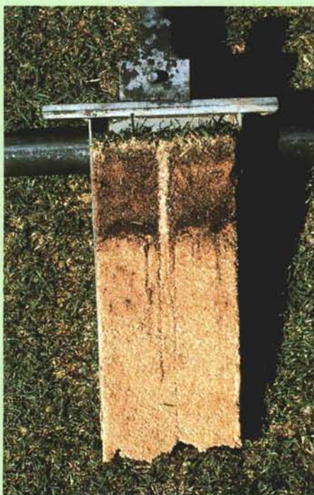
The grow-in layer on a pure sand green can cause layering problems that eventually lead to black layer.
