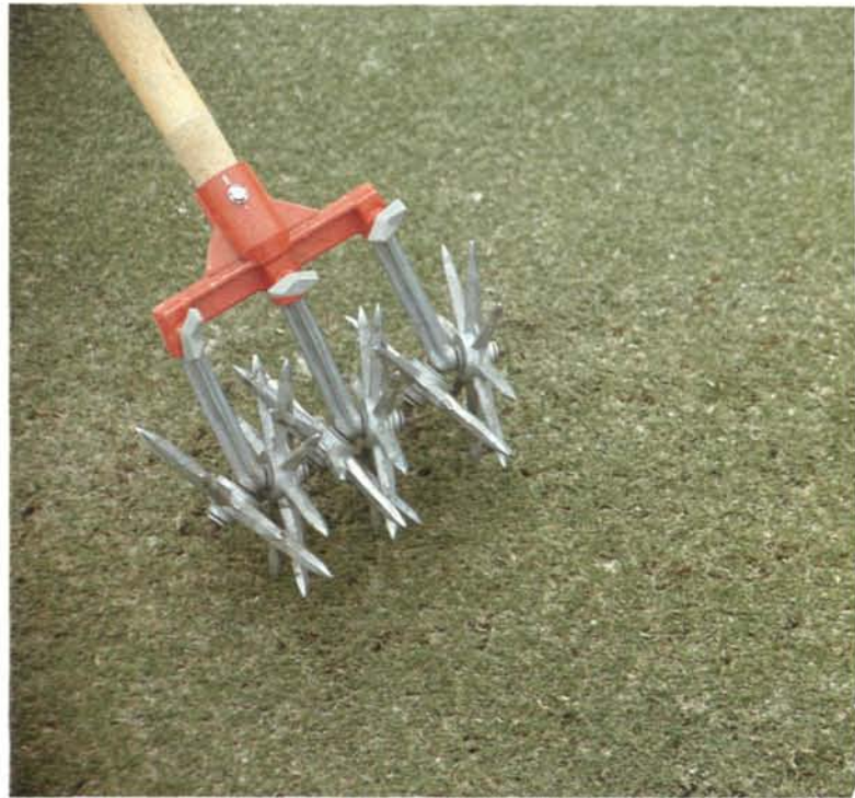
A groomer reel, mounted on a lawn mower handle, is one method to help the superintendent break up an algae layer (left). The Garden Weasel is being worked over a problem area, resulting in a thorough shredding of the algae crust (right).
