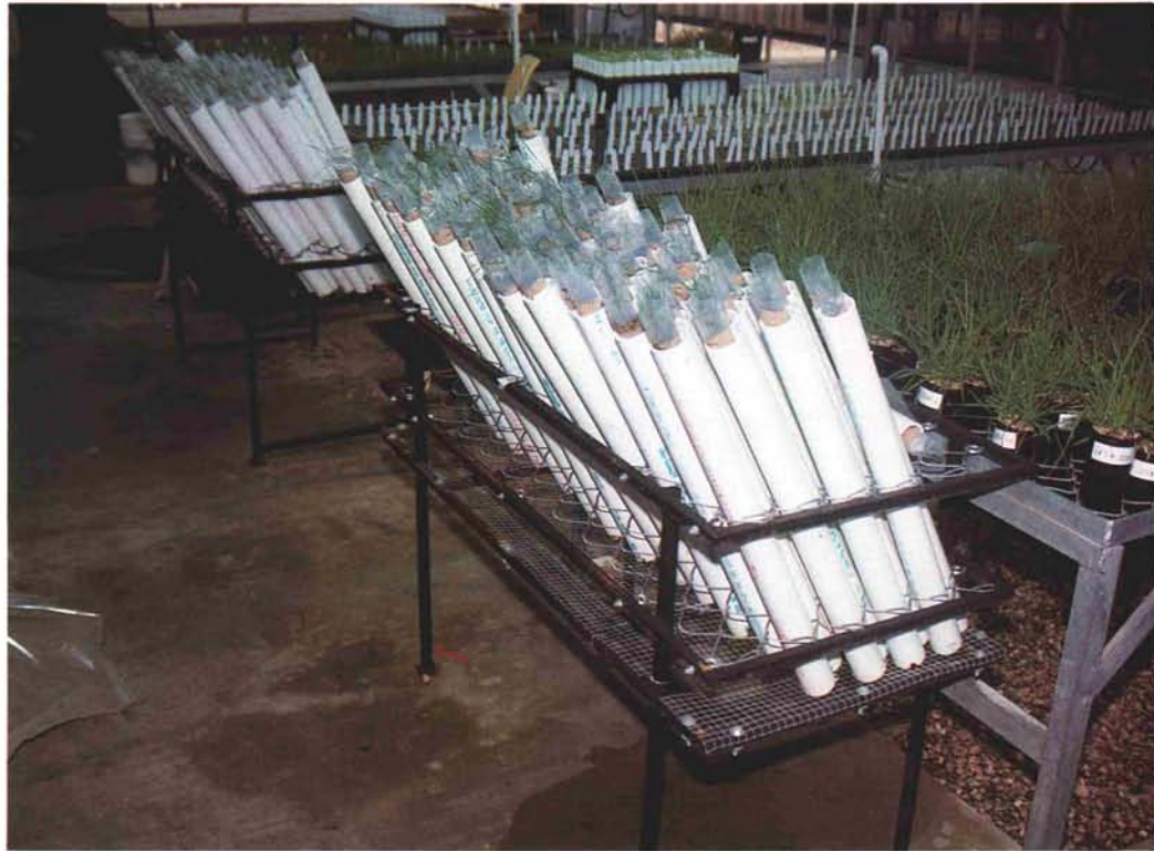
Root distribution influences the ability of the turf to access soil moisture reserves. Slanted root tubes aid in studying root distribution and rate of development.
