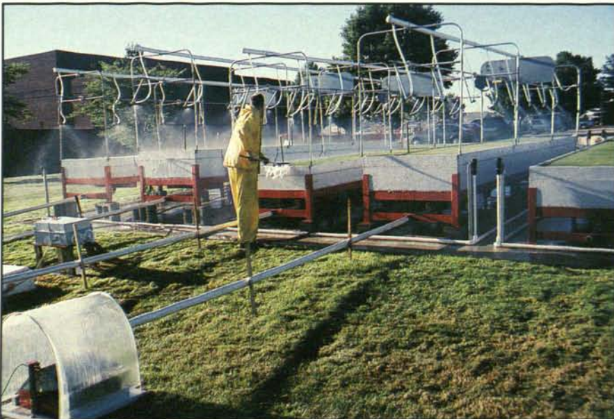
The research greens are constructed from 4-foot by 24-foot wooden boxes. The support legs are blocked for slope adjustment, rain simulators are located overhead, and tipping bucket rain gauges are attached to the drainage outflow lines to allow for the measurement of water output.
