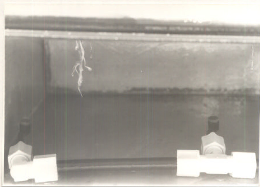
Figure 5. Mist nozzels enclosed in the tank showing how roots are misted with the salt solutions.
