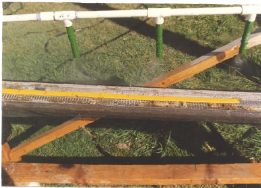
Figure 4b. Gentle mist washing of TRIF cores removes sand to enable distinction of root characters.
