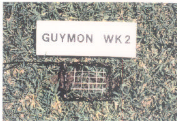
Fig. 6. A grid is used to measure recovery from divoting.
