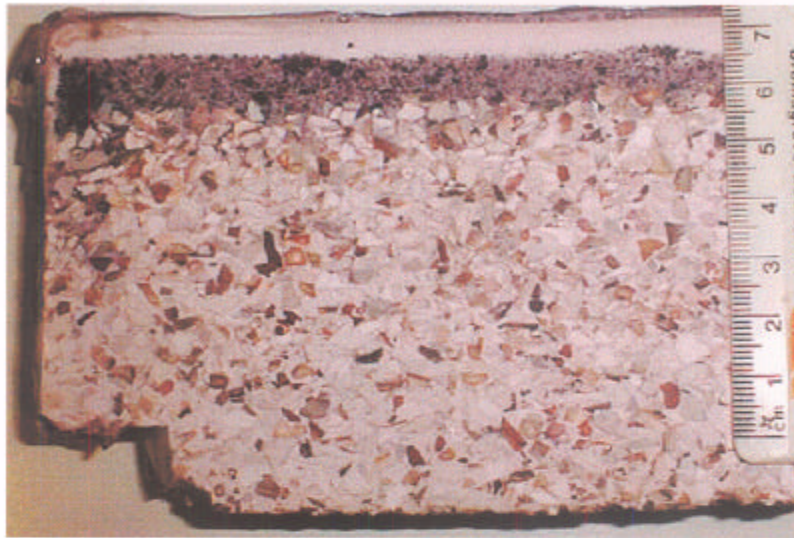
FIGURE 1. Profile of rootzone over fine gravel under normal light conditions (the rootzone/gravel interface can be seen running horizontally between 5 and 7 cm on the adjacent scale). No particle migration is evident.
